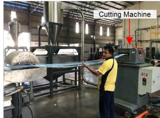
Feeding solidified plastic strands into a cutting machine.
