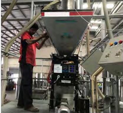
Loading raw materials into a dosing system.
