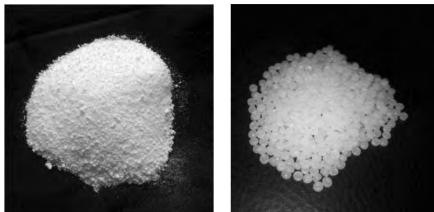
Plastic Powder (left) and Plastic Pellets (right)
