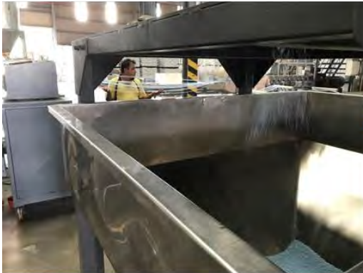
Collecting plastic pellets from the cutting machine.
