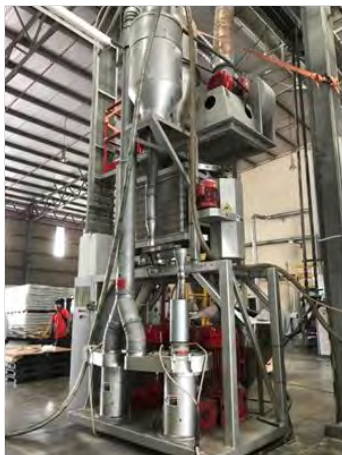
Attrition grinding mill in operation.
