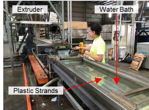
Cooling semi-solid plastic strands in a water bath.
