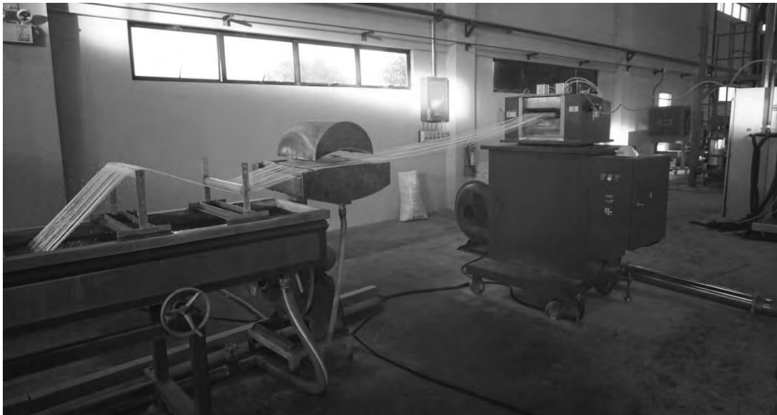
Cooled Plastic Strands and Cutting Machine at our Clark Freeport Factory
