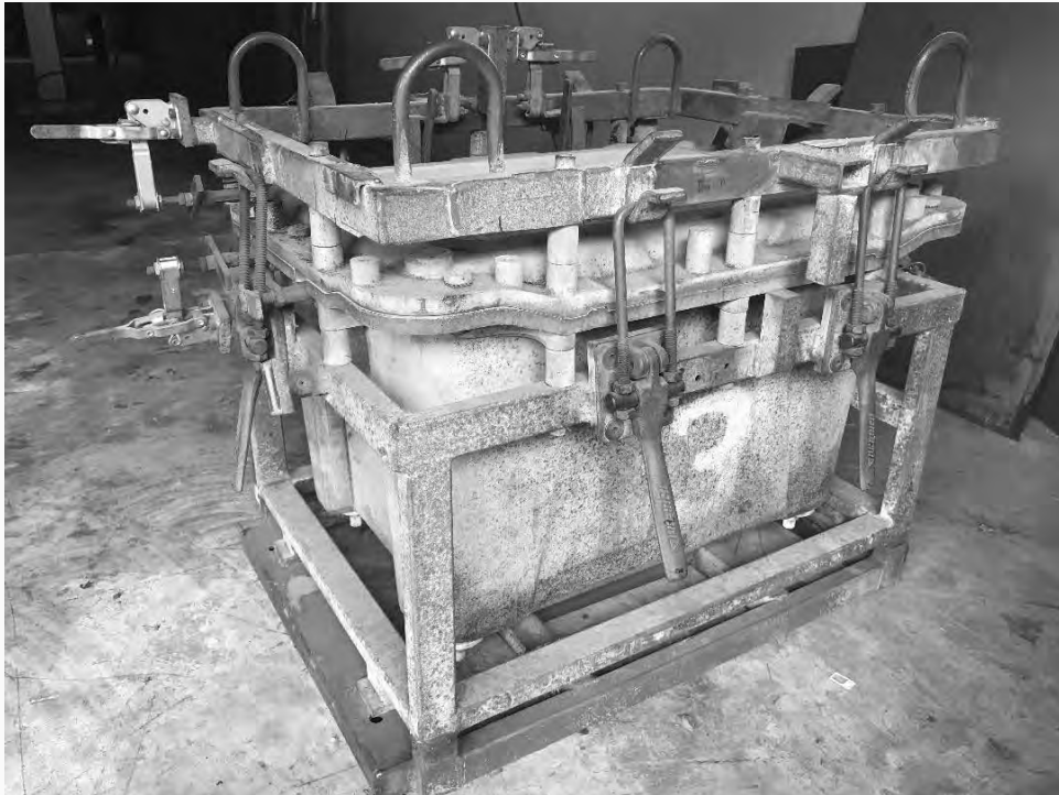
One (1) of our Moulds for Rotational Moulding
